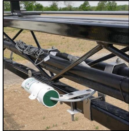
3. Pictures of the new sensor and housing. Housing style and mounting brackets allow more flexibility for positioning the sensor on the boom.
