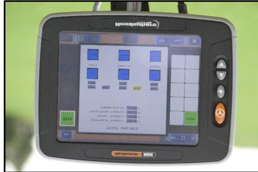
7. In the past, when new firmware upgrades became available, users had to return the Controller to Greentronics to have the new firmware installed. The new RiteHeight Controller contains a Bluetooth chip. Firmware on the RH430 Controller can be upgraded by obtaining the upgrade file from Greentronics and uploading it on the Controller via android App and Bluetooth connection between your smartphone or tablet and the RiteHeight Controller.
