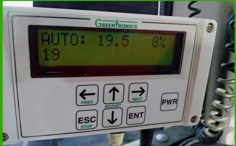
**Controller with sealed keypad and display to engage & disengage automatic mode and to navigate the menu system for set-up and diagnostics.**
