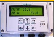
Controller Easy keypad allows engaging and disengaging automatic mode, as well as adjusting target depth on-the-go. The same controls are used to navigate the menu system.
