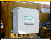
Interface Box The sensor(s) and solenoid wiring are all connected to the Interface Box, which connects to the Controller with one communication cable.
