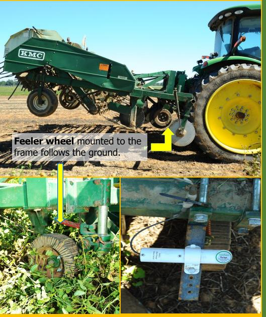
Sonar sensor mounted above wheel continuously measures vertical position of the wheel with respect to the frame. The Controller makes automatic depth adjustments to maintain the optimum.
