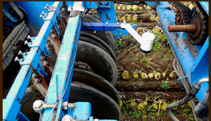
RiteDepth System on a Pearson 3-row Turnip harvester
