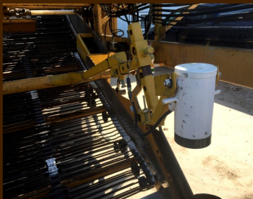
RiteDepth System on a 3-row KMC Peanut Inverter
