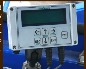
RiteDepth System on a Pearson 3-row Turnip harvester
