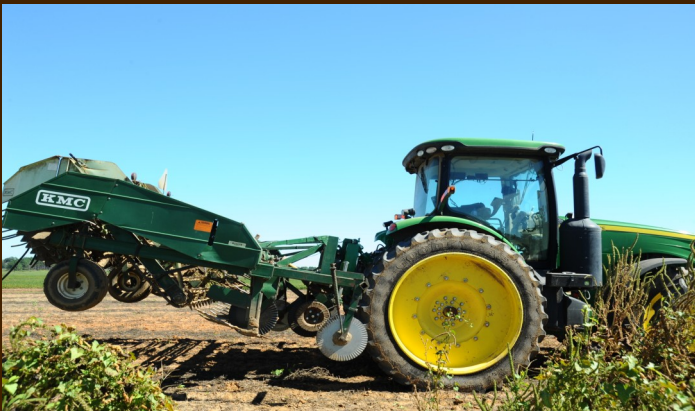
RiteDepth System on a 3-row KMC Peanut Inverter
